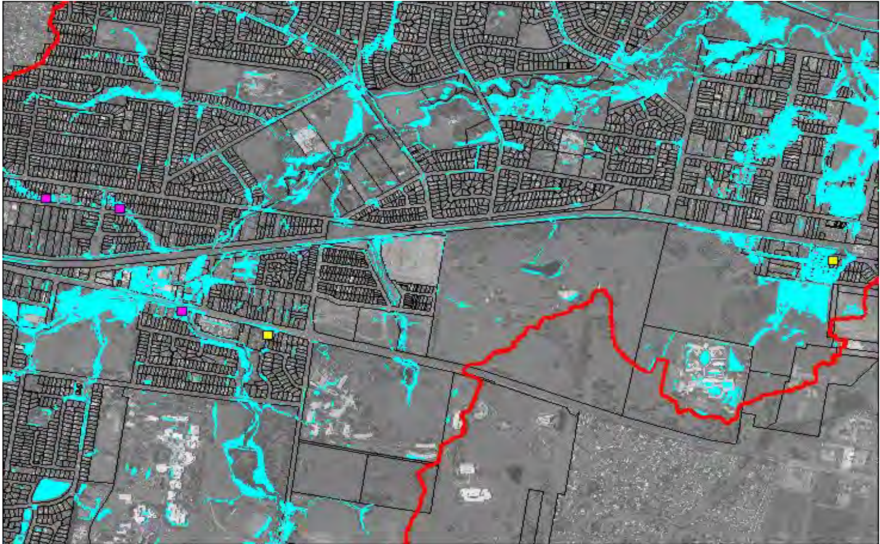
Plate 59 1% AEP low hazard areas (aqua) and properties potentially eligible for voluntary raising (yellow) or voluntary flood proofing (pink).
