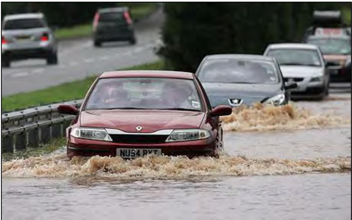
Plate G4 Example of cars driving through flood waters and generating waves
