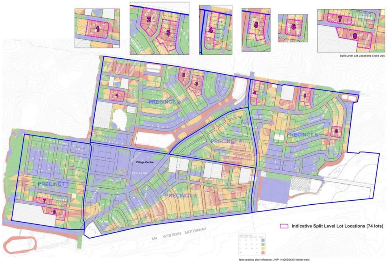
Figure 26 Indicative subdivision layout for slopes in excess of 10%
