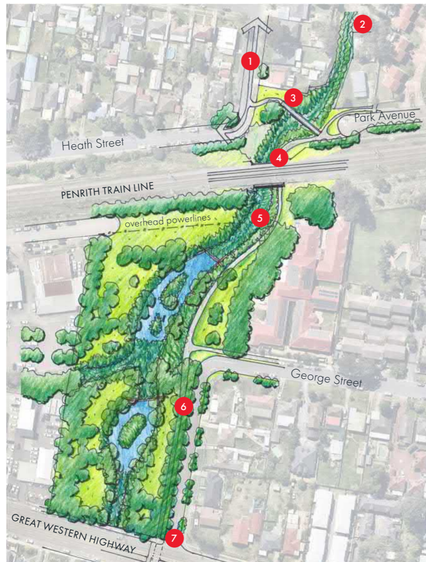
Figure 58. Concept Plan - Shared path connection and creek restoration to connect under train line to improve pedestrian link between Werrington and Kingswood
